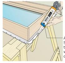
Apply MOISTOP SEALANT around the edges of the window nail fin covering ALL holes.
