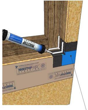
INSERT GS100'A' AND PRESS TIGHTLY. INTO CORNERS. APPLY SEALANT ON TOP OF GS 100'A' AS SHOWN
