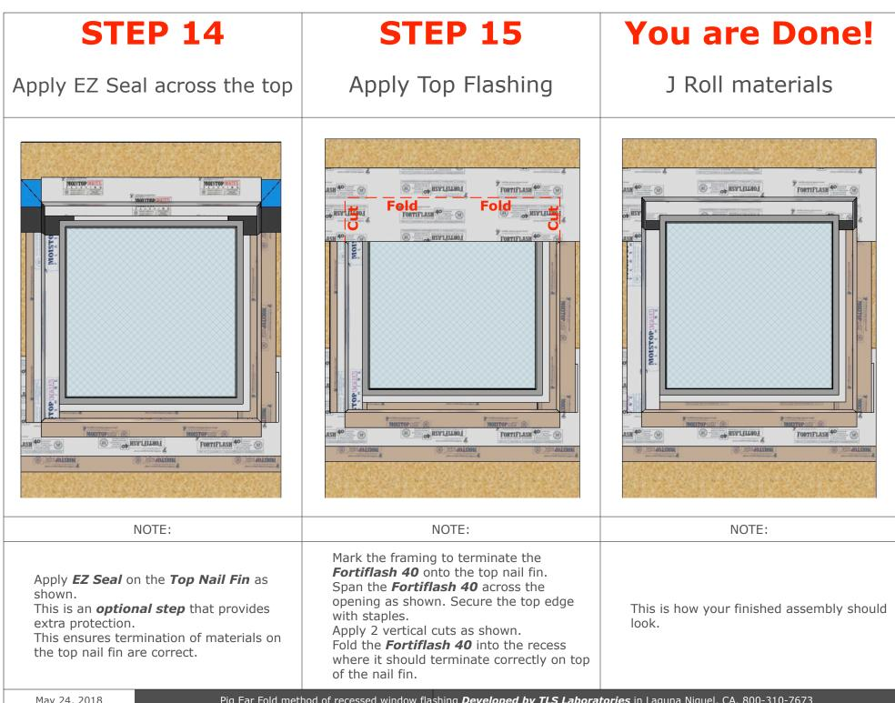
Pig Ear Fold method of recessed window flashing *Developed by TLS Laboratories* in Laguna Niguel, CA. 800-310-7673
